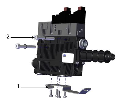
1 DIN rail mount for TS35 DIN rail, incl. plastic tapping screws Max. tightening torque 0.5 Nm 2x M4 fastening screws with washers
