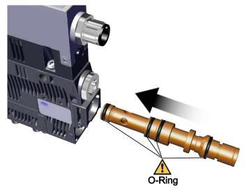
3. Install any cleaned or new nozzle in the correct position. Ensure that the O-ring is fitted.
