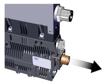
⇒ The nozzle is removed together with the Oring.
