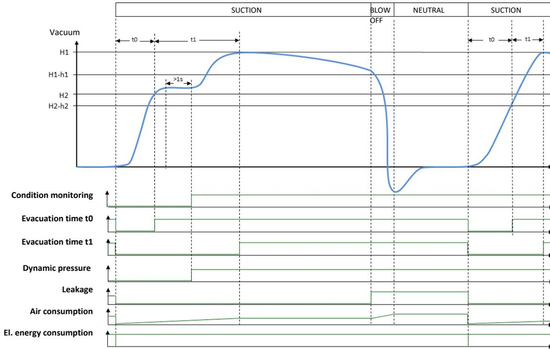
Handling cycle with leakage > L and readjustment:
