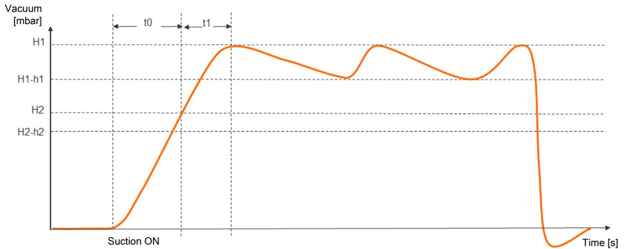
If the measured evacuation time  $t_1$  (from H2 to H1) exceeds the specified value  $[t-1]$ , the "Evacuation time longer than  $t-1$ " condition monitoring warning is triggered and the system status light switches to yellow. The specified value for the max. permitted evacuation time can be set under the  $[t-1]$  menu item in the configuration menu or via IO-Link. Setting the value to "0" deactivates monitoring. The maximum permitted evacuation time setting is 9.99 seconds.
