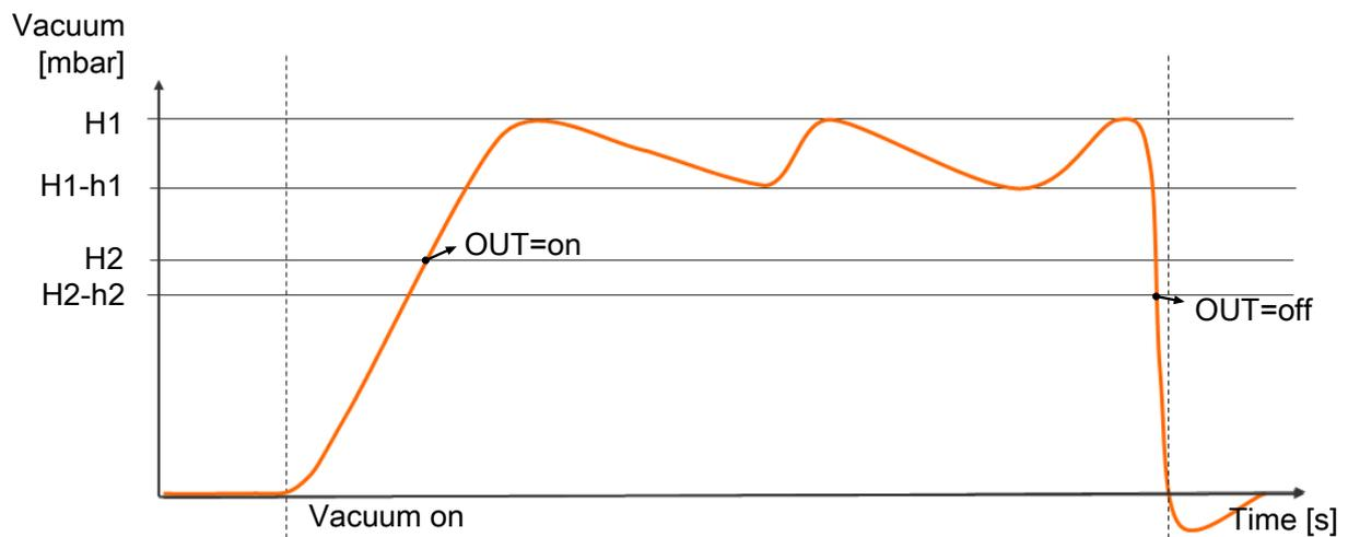
The ejector has an integrated air saving function and automatically regulates the vacuum in suction mode:
