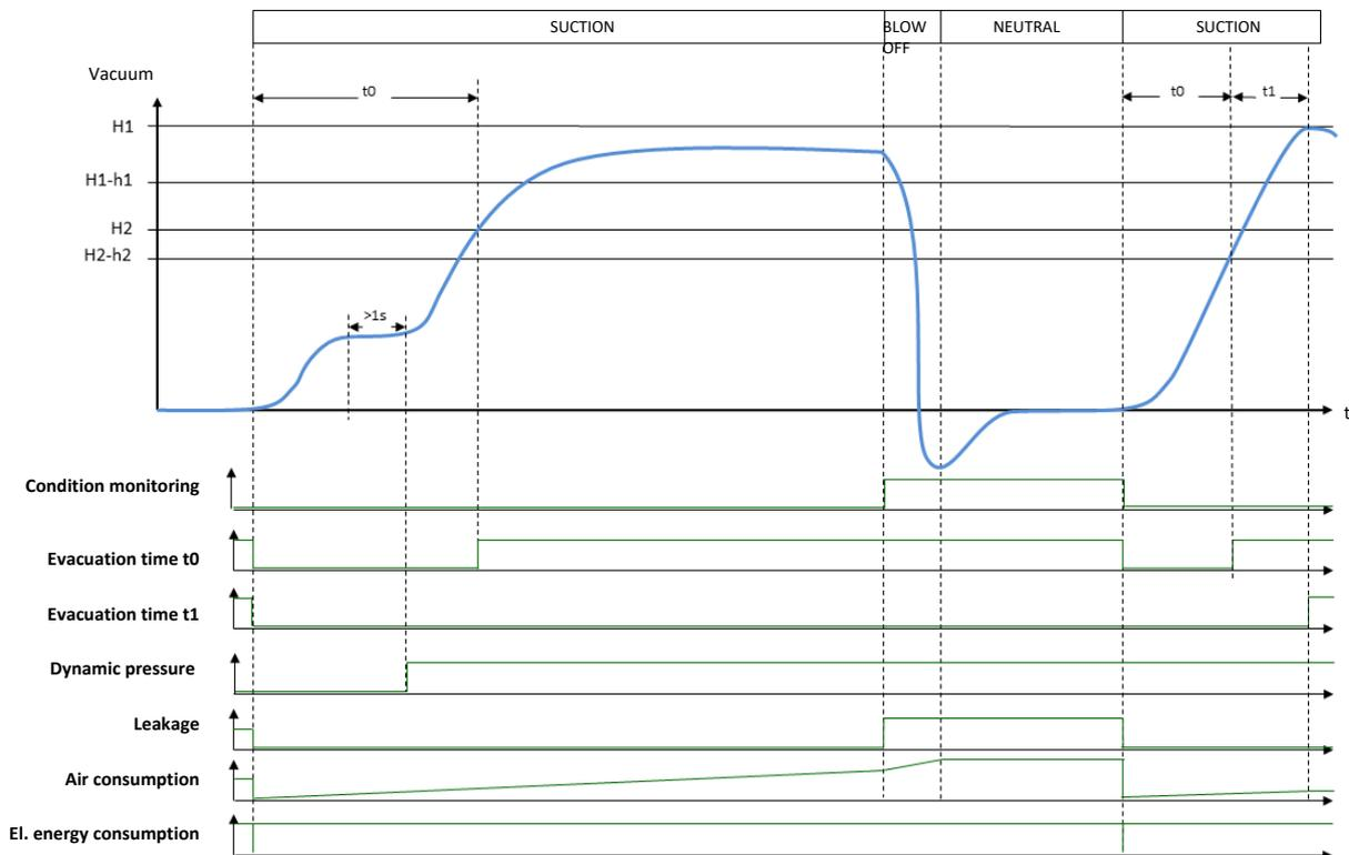
Handling cycle with excessive evacuation time  $t_1$ :
