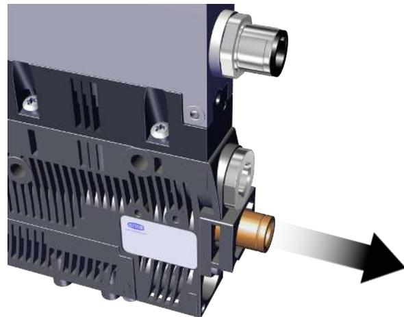
⇒ The nozzle is removed together with the O-ring.
