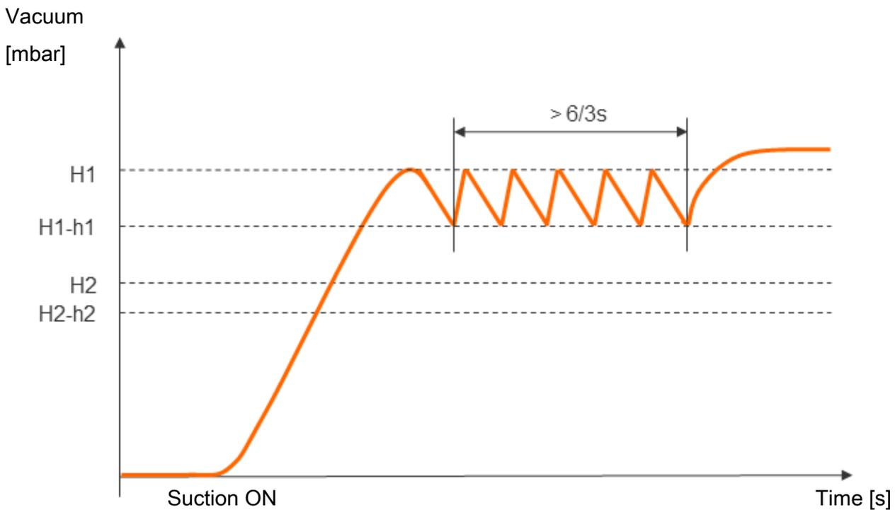
With the  $[dcs = 0h]$  setting, continuous suction is deactivated, and the ejector continues in control mode despite a high leakage rate or control frequency greater than 6 times per 3 s.
