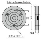
• When a key 1 is placed within the antenna detection zone, a signal is sent to the control unit to unlock the doors connected to it. The antenna can be mounted either inside or outside the cabinet.
