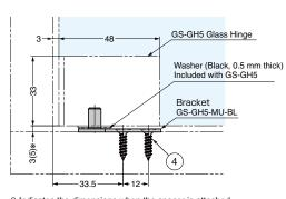
() Indicates the dimensions when the spacer is attached
