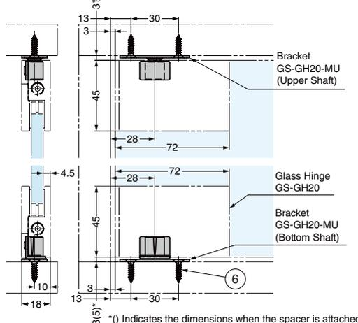
Sold in sets of an upper shaft unit, bottom shaft unit, and spacer.
