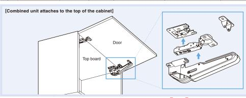
Simple installation only requires AILERON to be placed on OLYMPIA with a mounting plate  $% \left\{ 1,2,\ldots,n\right\} =0$ designed for AILERON
