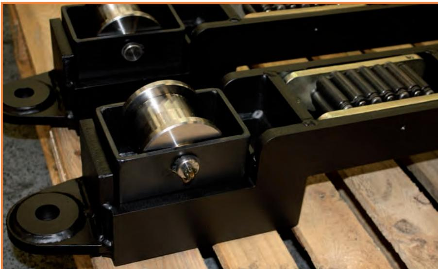
The bored tunnel of concrete section was 2.2m diameter and the gas pipe within this tunnel was 1.2m diameter leaving very limited space between the two, so the gas pipe supporting trollies had to be small enough to enter this gap between the pipe and the tunnels walls but have very high loading capacity to take the gas pipe as it was pulled/pushed into the outer tunnel. The rail system for the trollies was laid on a bed of silicon sand.
