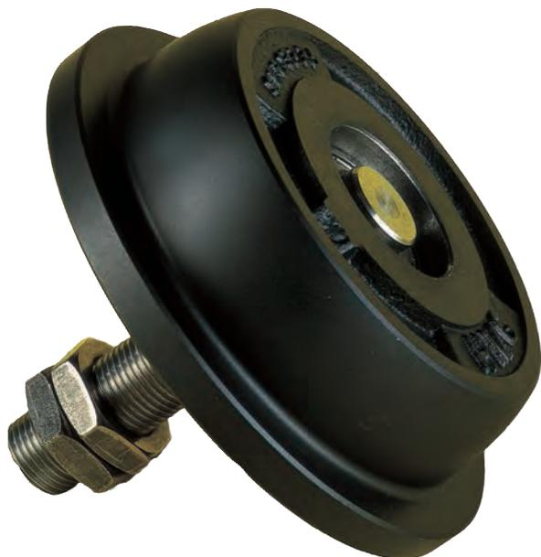
The SFR (cast iron) and SSFR (Steel) ranges of wheel assemblies have been designed to fit within standard sections of channel and 'I' beams. The radiused tread accommodates the angle of the section and improves the wear and tracking characteristics.
