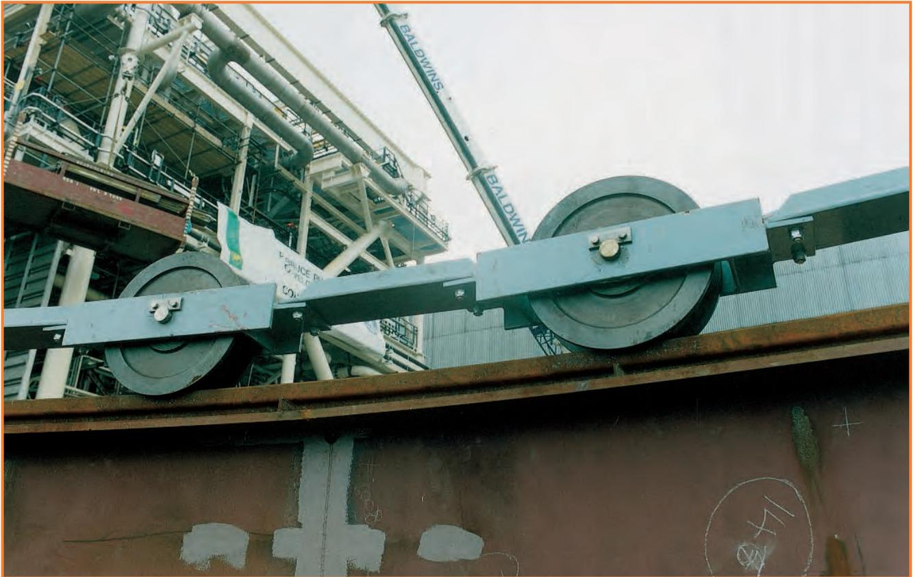
7600 tonne, 32 meter diameter, pipe laying turntable running on 330 steel double flange rail wheels fitted with self-lubricating bushes and stainless steel shafts.
