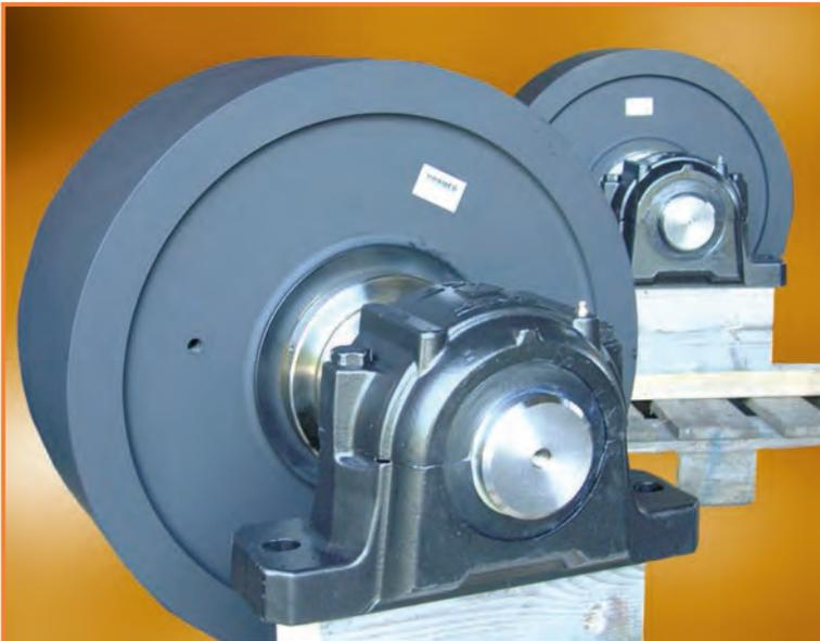
Wheel and axle assemblies used in a rotating drum application. Given the extreme conditions and high loadings involved the wheels and axles have been specifically designed to the customers requirements that demand flat tread wheels with axles that are capable of taking a load in excess of 75 tonnes.
