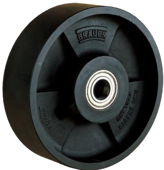
Untyred wheels can carry high loads with low rolling resistance when used on a hard surface such as flat steel. On softer surfaces, such as concrete or tarmac, the surface is likely to be worn or indented by the use of an untyred wheel. Untyred wheels are noisier in operation than tyred wheels, but noise is unlikely to be a problem at walking speeds.
