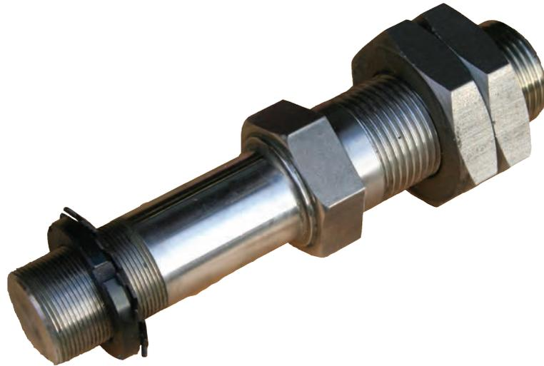
This range of cantilevered stub axles is designed to mount single wheels with ball or roller bearings, the lock nut and lock washer, or self locking nuts providing adjustment for opposed taper roller bearings.
