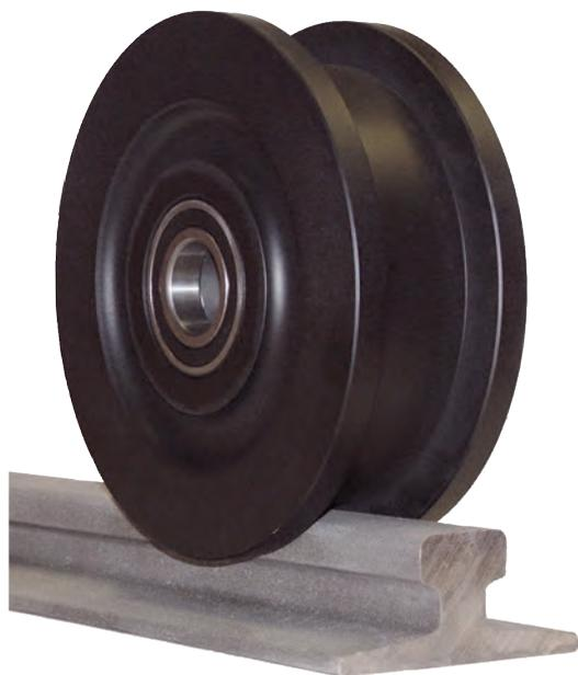
Cast iron rail wheels are the most economic for light to medium duty, but they have a limited service life when compared to steel wheels, and are unsuitable for high rotational speeds or where substantial shock loads are to be withstood.
