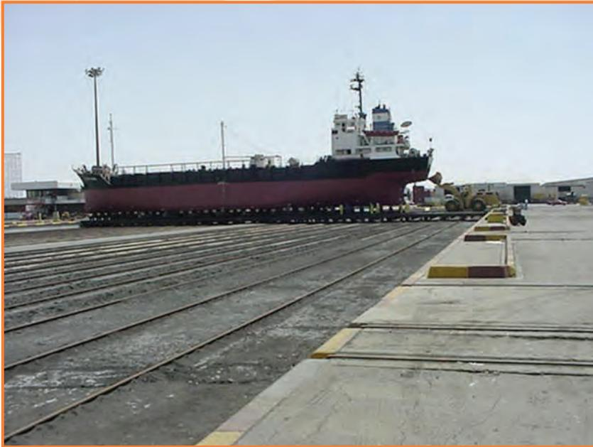
A ship lift and transfer dock system for removing ships from the sea and then transferring ships around the dock for repair and maintenance to take place. Three sizes of wheels are used throughout the dock.
