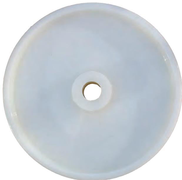
Plain untyred nylon wheels are the least expensive type of wheel. They are light in weight, and are resistant to impact, abrasion, corrosion, and the effect of many chemicals. They can be fitted with bearings but are most often used with their nylon bores running on a smooth steel axle. No lubrication is necessary, but they will benefit from being oiled. Having little resilience they tend to be noisiest when moving quickly over rough surfaces, and they can mark floors if highly loaded.
