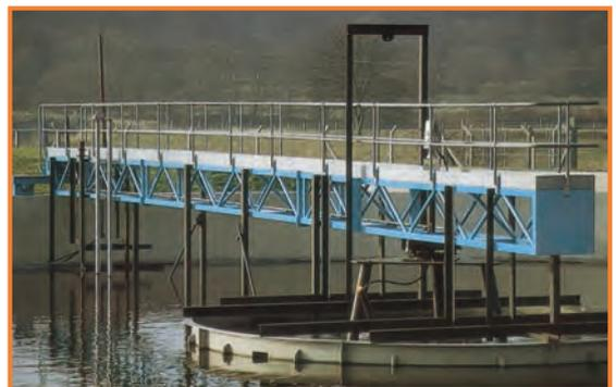
*Half Bridge scraper for rotary settlement tank*
