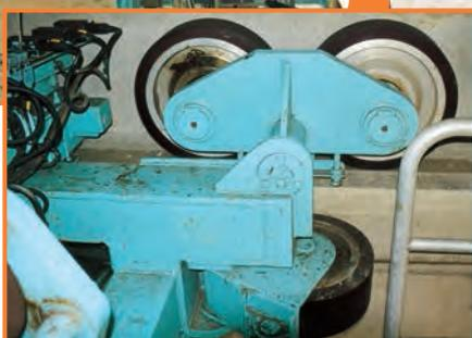
Polyurethane tyred wheel fitted with spherical roller bearings. Tread diameter 500mm. Tread width 100mm. Maximum radial load capacity 50KN. Tyre 95-98 Shore 'A' hardness directly bonded to aluminium grade BS1471-6082-T6 centre to significantly reduce the weight for ease of handling. Aluminium anodised to prevent corrosion.
