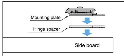
Set the spacer between the mounting plate and side board.
