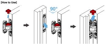
\*Please do not detach the jig until the hinge is installed.
