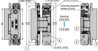
\*The upper screw covers are removed in the drawing above.
