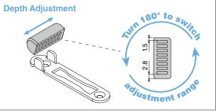
Allows for 4-level depth adjustment by changing the slits to insert. When turned 180°, additional 4-level adjustment are available. (Total 8-level)
