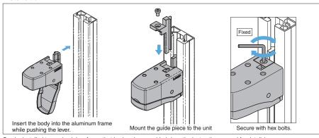
Can be installed to an aluminium frame that is already assembled. (see the instruction manual for details)
