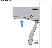
Open the cover and push the lever to move the unit up or down. The unit stops where the lever is released.
