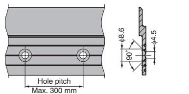
Mounting holes should be located symmetrically to the centre of mounting surface, with the pitch below 300mm.
