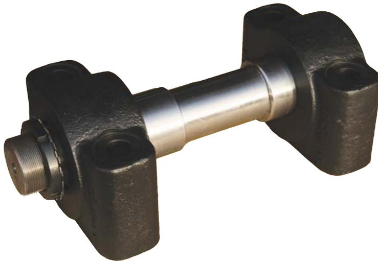
The 'BA' series axle assemblies are for mounting single wheels fitted with ball or roller bearings, the lock nut, lock washer, or self locking nuts and sleeve providing adjustment for opposed taper roller bearings.
