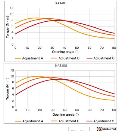
The indicator shows how much balance-adjustment is applied. Balance-adjustment should depend on the location of the center of gravity. When used in:
