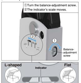
The indicator shows how much balance-adjustment is applied. Balance-adjustment should depend on the location of the center of gravity. When used in:
