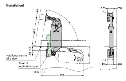
\*The Max. door moment depends on location of center of gravity, installation point of stays, and balance adjustment.
