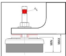
4. Level the machine by acting on the hexagon at the top of the screw. The disk will raise
