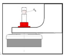
3. Apply the nut/washer and tighten it.
