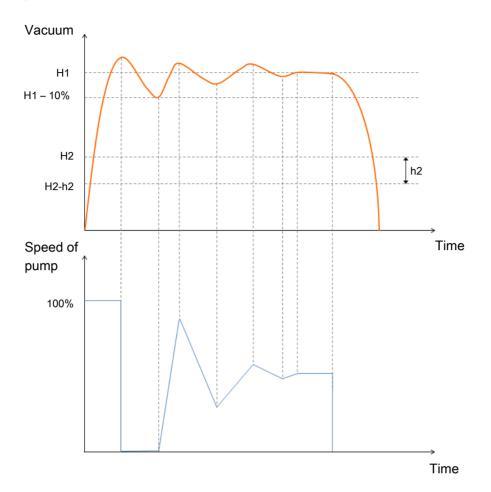
The output OUT2 (parts control) is set to "on" when the limit value H2 is reached. If the limit value H2-h2 is underrun, then the output is set to "off."
