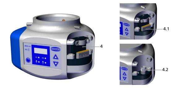
The CobotPump is electrically connected to the power supply and for input and output signaling purposes via the interface at item 4. The connection can be established using a flexible cable connection for device versions with a terminal block (4.1) or an 8-pole M12 connector (4.2).
