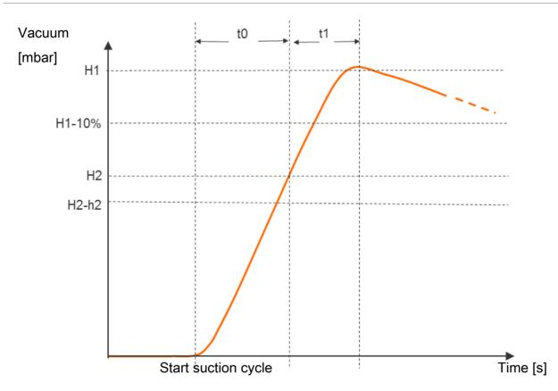
The specified value for the max. permitted evacuation time can be set in the configuration menu with the parameter [b - 1] or via IO-Link [0x006B]. Setting the value to  $[\Box \Box \Box]$  (= off) deactivates monitoring. The maximum permitted evacuation time setting is 9.99 s.
