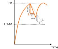
The permitted leakage value -L- can be set in the configuration menu with the parameter [-L-] or via IO-Link.
