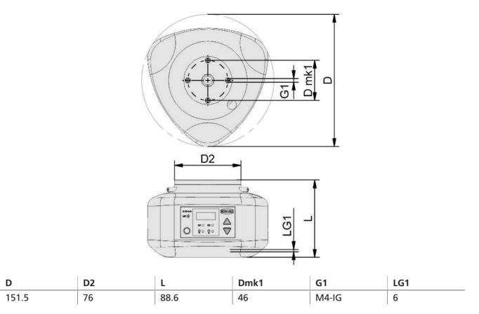
All dimensions given in millimeters [mm]
