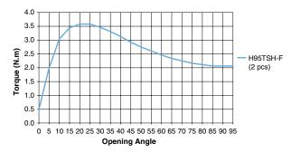
Although the torque will be released to prevent "spring-back" at a nearly closed angle, the door will not be firmly kept closed. If detent function is needed, please use with catches.
