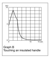
The y-axis represents the natural voltage of the human body (in kiloVolts), and the x-axis represents elapsed time (in seconds). Contact with the hardware occurs at the 4 second mark.
