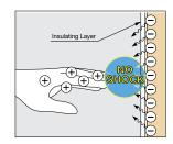
In the figures above, a human hand with a positive charge is approaching a conductive surface with a negative charge (e.g., metal). The figure on the right incorporates a layer to insulate the discharge.
