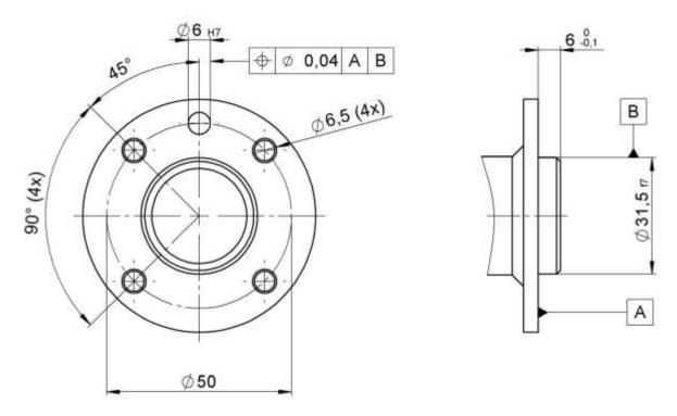
The gripper initially comes equipped with a Ø31.5 f7 base in the corresponding robot flange adapter in order to mount the gripper onto the robot/system.
