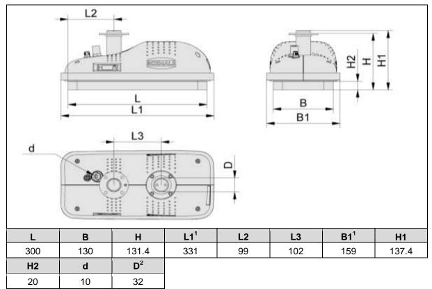
Exact dimensions vary based on the circumferential foam <sup>2</sup> Only for the FMCB
