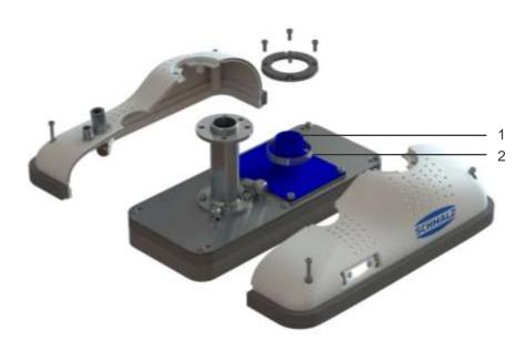
A hose that is suitable for vacuum applications must be connected at the installed hose connection and secured with the included hose clamps. The supply hose must have the same nominal diameter as the installed connection. The maximum recommended hose length is around 10 meters. For instructions on opening the housing, see chapter 8.7.
