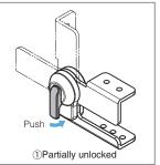
The flap is temporarily unlocked while the lever is pushed.
