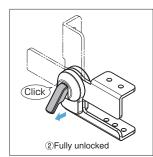
The flap stays unlocked when the lever is lifted.
