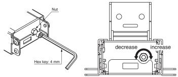
①Loosen the nut of adjustment screw.
