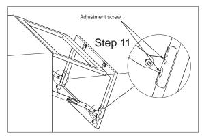
Fig. 10 Adjustment screw in detail
