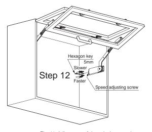
Fig. 11 Adjustment of door closing speed
