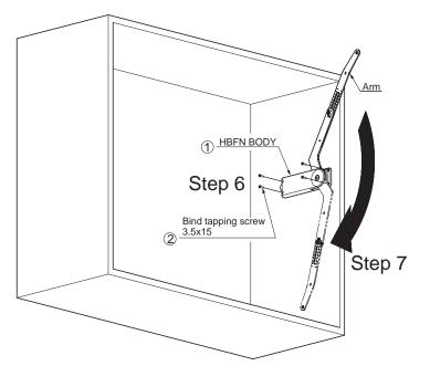
Installation of HBFN unit body
