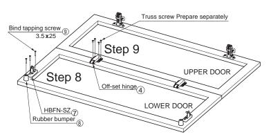
Fig. 8 Installation of HBFN-SZ mounting plate and off-set hinge
