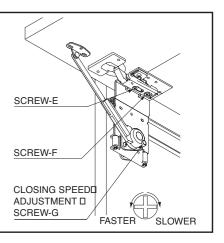
This product is designed as a soft-closing stay and slide mechanism for a inset opening flipper door. We shall not be liable for any injuries or damage to the product due to incorrect installation and
