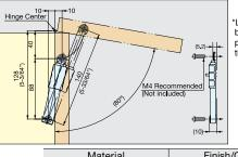
\*Lid stay must be installed parallel to the sidewall.
