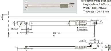
A, B and C dimensions are for 90° door opening angle
