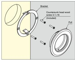
Please insert the pull after installation of the bracket with screws. (This picture refers to ZL-2501-56)
