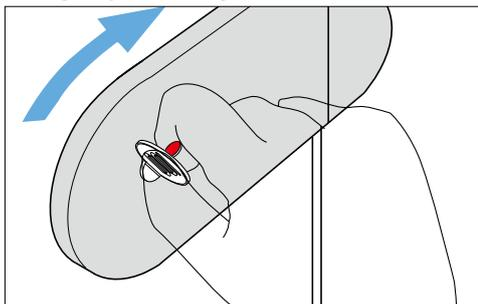
The indicator has a feature which enables unlocking the door from outside in an emergency. To unlock, rotate the centre 90° with a coin, etc. as shown in the figure above.
