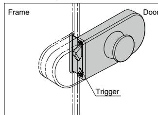
The trigger senses whether the door is open or closed, and only enables the thumbturn to be turned all the way when the door is closed.
