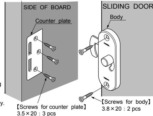
\*If you have a recess mounting application, please cut out a section out of the slide board section for the latch hook before mounting the counter plate.
