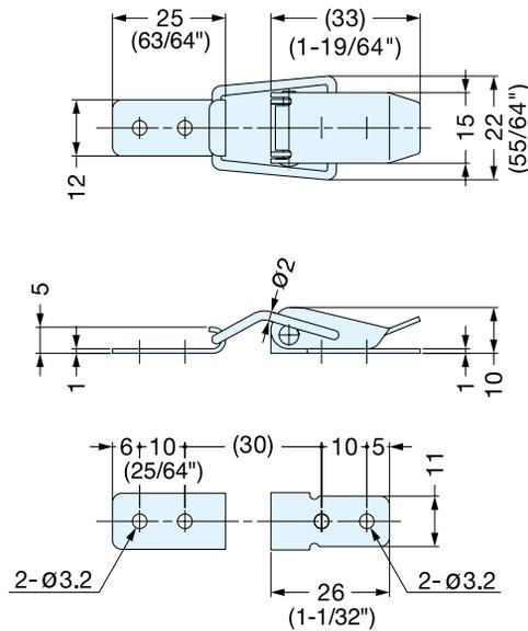
\*Dimension shown is in case of clamping force "0.5".
