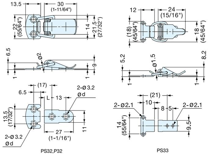
\*Dimension shown is in case of clamping force "0".
