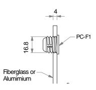
PC-F1 can be used as screw / friction fit into thin frames & seat backs
