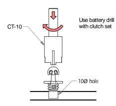
INSTALLING ADHESIVE FIT MALE CLIPS (first complete steps 1 to 3, page 1)
