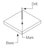
Screw on TC-M6 to base using #6 gauge CSK screw
