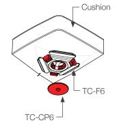
Press cushion into place, pushing down on clips firmly to mark base
