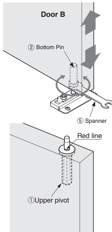
Check if the red line on the pivot is hidden or not. If it is visible, rotate the pivot on the bottom pin to raise the door.
