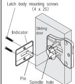
Insert the pin of the indicator into the spindle hole at the center of the latch body, and use the latch body mounting screws (4 x 25) to mount the indicator to the latch body. (At this time, set the color of the indicator window to blue .)
