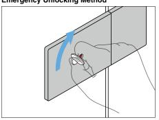
The indicator has a feature which enables unlocking the door from outside in an emergency. To unlock, rotate the centre 90° with a coin, etc. as shown in the figure above.
