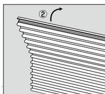
Install the profile ② until it reaches required height. The profile will cover the screws.
