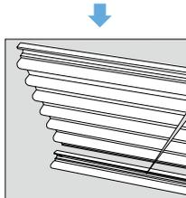
Install the bottom rail ①. Level the bottom rail before fastening. Insert the profile ② into the bottom rail. Fasten with screws.
