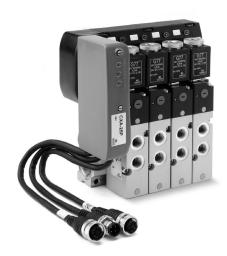
In the Multipole version the front position of the 25 pin Sub-D connector makes the connection easier. The connectors with prewired cable, which are available in different lengths and with axial or radial orientation, simplify the electrical connection. The Island can be configured up to a max. of 22 solenoids, using monostable and bistable electrical modules, on 22 valve positions, for example 22 monostable solenoid valves.
