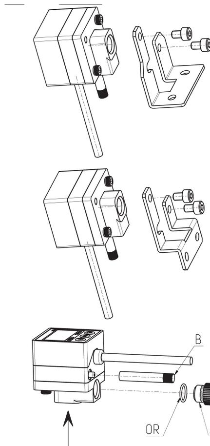
**Example of mounting with panel mounting set Mod. SWCN-F**
