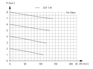
Pa = Inlet pressure - Pr = Regulated pressure
