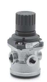
Series N pressure regulators are available with G1/4 and G1/8 ports. Their design incorporates a self relieving diaphragm so as to allow decremental adjustments.
