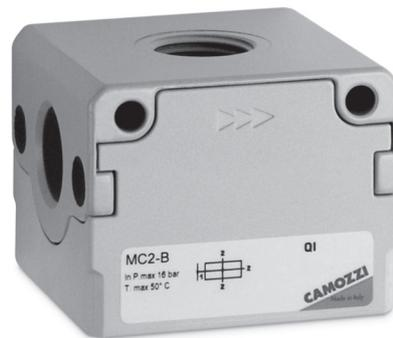
The take-off blocks, when equipped with a no return valve, allow the use of non lubricated air and should be inserted between the regulator and the lubricator. If mounted as last element, they should be assembled with terminal flanges.
