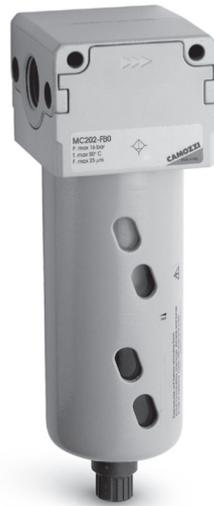
Series MC coalescing filters are available with G1/4, G3/8 and G1/2 ports. The bowls of these filters are made of metal with a transparent sight glass and may have a condensate drain valve which can provide either a manual or semi-automatic function.
