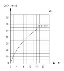
RFU 452-M5: flow from 2  $\rightarrow$  1 needle type OPEN = 55 NI/min CLOSED = 41 NI/min
