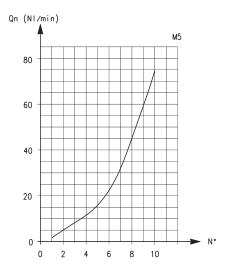
To ensure the right choice of unidirectional flow controller, proceed as follows: calculate the quantity of air in NI/min (see cylinder Table); determine the stroke time of the cylinder; refer to graph to see which controller is the right type.
