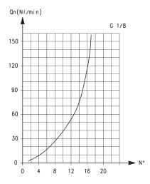
Flow Qn (NI/min.) from  $2 \rightarrow 1$  with controller OPEN: 70 Flow Qn (NI/min.) from  $2 \rightarrow 1$  with controller CLOSED: 33
