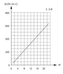
Flow Qn (NI/min.) from  $2 \rightarrow 1$  with controller OPEN: 530 Flow Qn (NI/min.) from  $2 \rightarrow 1$  with controller CLOSED: 160 Flow Qn (NI/min.) from  $2 \rightarrow 1$  with controller OPEN: 710 Flow Qn (NI/min.) from  $2 \rightarrow 1$  with controller CLOSED: 410
