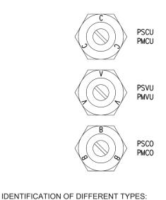
PSCU - PMCU = assembly directly on the cylinders PSVU - PMVU = assembly directly on the valves PSCO - PMCO = assembly directly on the cylinders or valves
