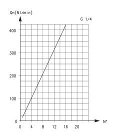
Flow Qn (NI/min.) from 2  $\rightarrow$  1 with controller OPEN: 200 Flow Qn (NI/min.) from 2  $\rightarrow$  1 with controller CLOSED: 70
