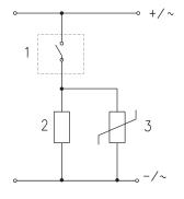
DC and AC applications: there is no protection on the Reed sensors on the inductive load, therefore it is advisable to use an electric ciruit with protection against the voltage spikes. See picture above for a typical example.
