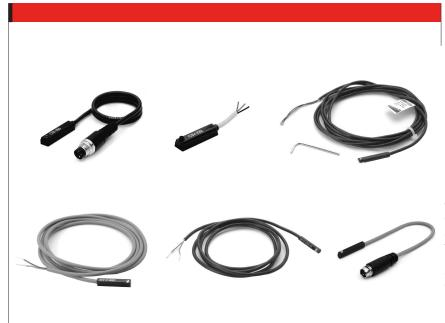
The magnetic proximity switches define the position of the cylinder piston. When the internal contact is actuated by a magnetic field, the sensors complete an electrical circuit and provide an output signal to actuate directly a solenoid valve or a PLC. A yellow or led LED diode shows when the internal magnetic contact is closed.
