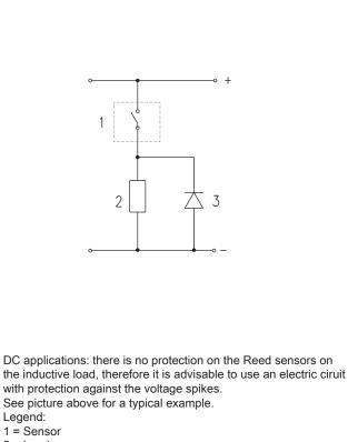
Electric circuit with protection against voltage spikes
