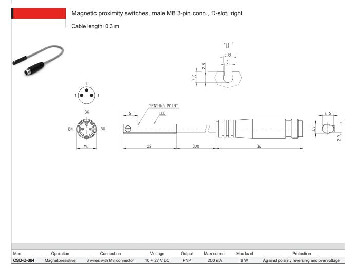
Magnetic proximity switches, male M8 3-pin conn., D-slot, 90° Cable length: 0.3 m
