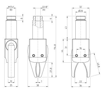
A = connection port B = fixing thread
