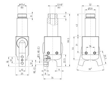
A = connection port B = fixing thread C = fixing holes
