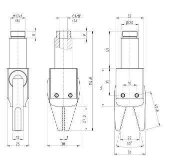
A = connection port B = fixing thread
